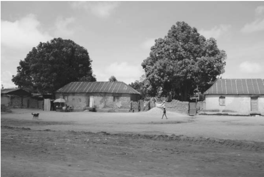
Mud-brick houses typical of rural architecture. Some are cement plastered and roofed with corrugated iron-sheets. Untarred roads that become muddy during rain also define rural setting. Courtesy of Armando J. Rodriguez, Jr.
